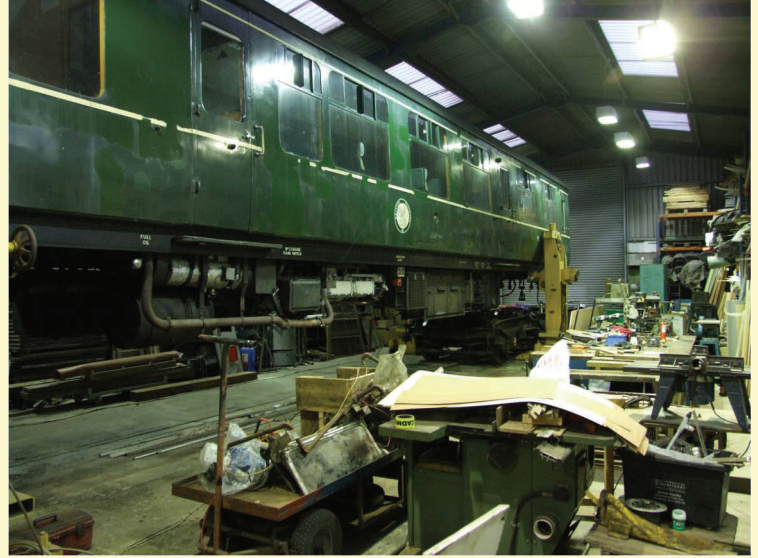
M50455's first preservation lift to enable bogie, brake and air tank work
